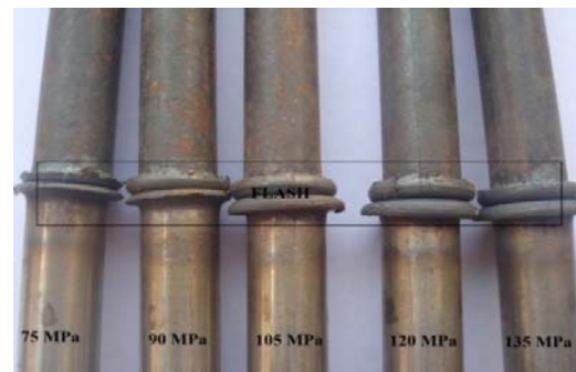
Fig. 1: Represents the Friction Welded Specimen at Different Axial Pressures Welded at 1120 rpm
