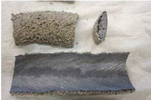
Fig. 1: Submerged Arc Welding Slag
