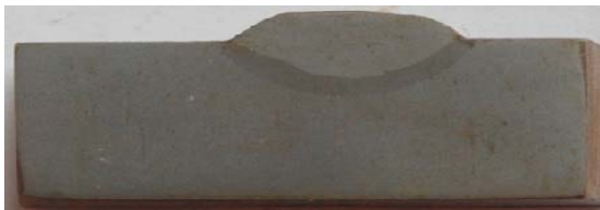
Fig. 4(b): Weld with Fresh Flux
