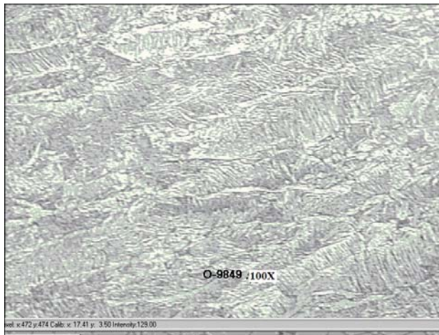
Fig. 7: Microstructure of Weld Metal Deposited with Crushed Slag (100X)
