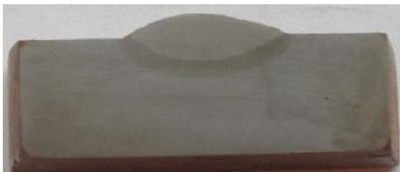
Fig. 4(a): Weld with Crushed Slag
