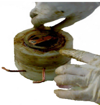
Fig. 2: Nylon Fixture with Copper Electrodes
