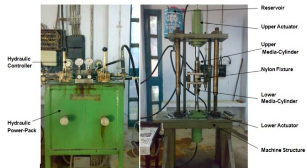
Fig. 1: Developed AFM Setup
